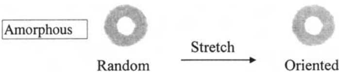
Figure 3.3 X-ray Diffraction Patterns as a Result of Orientation of an Amorphous Material
